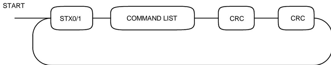
STX alternates between STX0 and STX1. Good messages are responded to by ACK0 or ACK1 the ACK matching the STX. If no ACK is received the message must be sent with the same flavour of STX. By this means lost ACKs do not cause message duplication.
